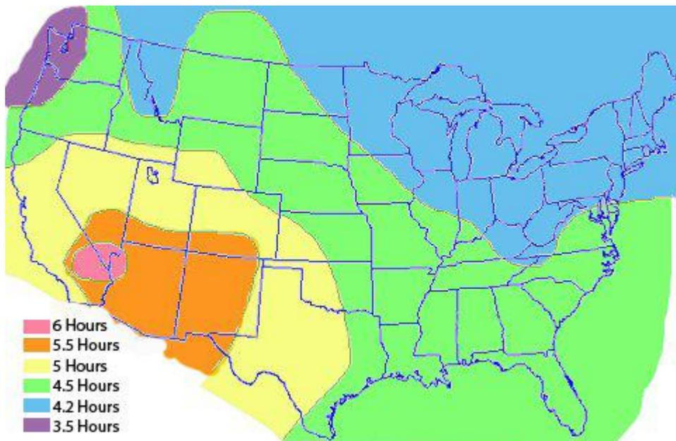
For instance, if you live in a place that gets an average of 4.5 hours of sunlight per day (most of the Midwest and South), your solar panel needs to be big enough to deliver 120 Watt-hours of electricity to the battery in 4.5 hours, which means it must be capable of delivering  $120/4.5 = 27$  Watts of electricity.
